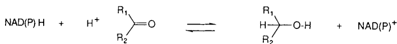
FIGURE 1 Generalized reaction catalyzed by hydroxysteroid dehydrogenases. R_1 and R_2 are components of either the steroid nucleus and/or side-chain.
